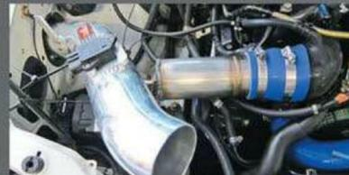
It can be a very good idea to make/use an intake leak test on any engine, regardless if the vehicle is boosted or simply naturally aspirated. To test for any leaks we constructed a homemade boost leak tester using a 2½-inch pipe welded on one side with a built-in nipple. To begin the testing process, we began by cooling off the engine before removing the intake filter to insert the pipe coupler.
