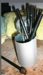
To test if a soda's acid can truly dissolve rust, we gathered up a set of used head studs from an old Subaru EJ20 engine sitting around in the garage. The head studs were heavily oxidized with rust and residue.
