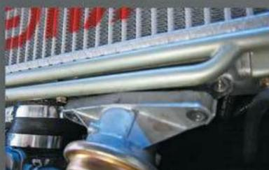
Listen for any hissing noise—this will indicate a boost leak. If the air pressure gauge indicates no buildup of pressure or does not hold for less than a second, that's a sure sign that a major leak exists within the engine. Be sure to pay close attention to problematic areas such as the blow-off valve or intake manifold for any leaks.
