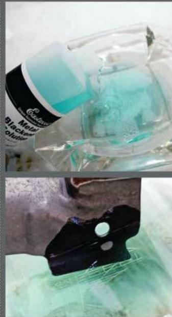
This chemical is odorless, non-caustic, and produces no fumes, making it safe for usage in and around the garage. Keep in mind this is not a paint product; the blackener is an etching solution.
