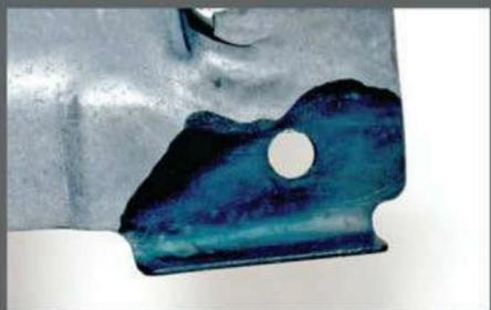
Once the part is clean of any rust and paint, it is then submerged into the solution for anywhere from 20 seconds to a minute (depending on surface area) as the chemical turns the metal from silver to black. After blackening, rinse the part in clean tap water for 10 to 20 seconds, and dry and wipe the surface with a clean cloth. Applying either a clearcoat or Eastwood's Diamond clear satin will help to maintain a rust-free finish.
