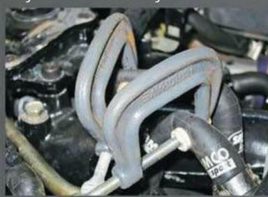
Be sure to seal any vacuum lines or hoses coming off of the intake pipe. If there's a PCV hose coming off the valve cover that connects to the air intake, plug the end that's on the air intake off. This also includes the vent crankcase pressure line.
